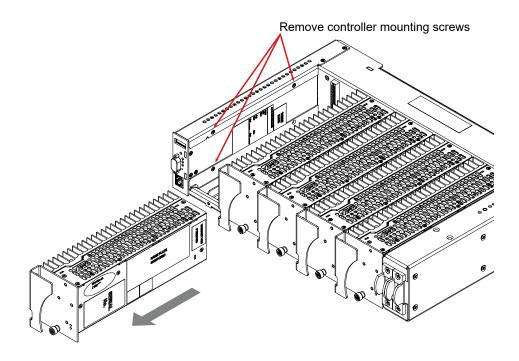
3. Pull from the location noted in the following image to remove the controller.
